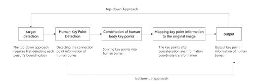
Fig. 2. The difference between top-down approach and bottom-up approach.
